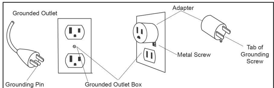
Whenever the adapter is used, it must be held in place by a metal screw.
