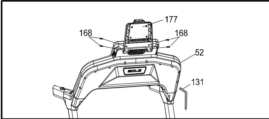
1. Insert Tablet Holder (177) into the Console Assembly (52) and use Combination M5 Allen Wrench & Phillips Head Screw Drive (131) to tighten four of Sheet Metal Screw (168).
