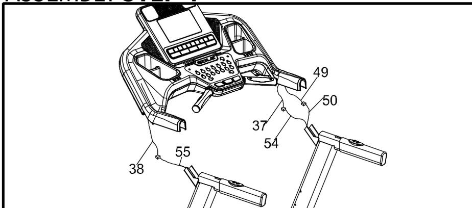
To complete this step, it is recommended that you find something to rest the console on at the appropriate height or have someone hold the console while you connect the cables
