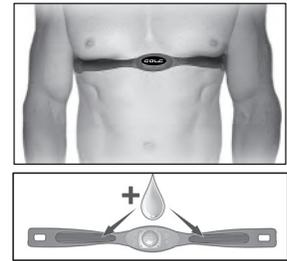
**Note:** The transmitter is automatically activated when it detects activity from the user's heart. Additionally, it automatically deactivates when it does not receive any activity. Although the transmitter is water resistant, moisture can have the effect of creating false signals, so you should take precautions to completely dry the transmitter after use to prolong battery life (estimated transmitter battery life is 2500 hours). The replacement battery is Panasonic CR2032.
