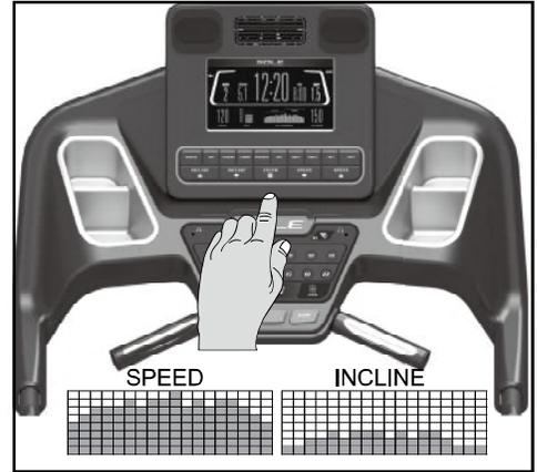
You may switch the speed or incline dot matrix profile shown by pressing the **Enter** button. Pressing the **Enter** button a second time will switch it back to the previous profile. Pressing it a third time will automatically alternate the Speed and Incline profile views.
